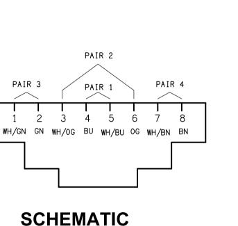
**RJ45 PINOUT CONFIGURATION**
